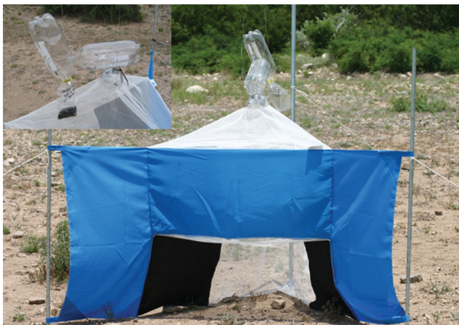
Figure 2. Unbaited Nzi fly trap setup. Flies enter through the opening between the black patches, fly upward toward the light, and get trapped in the bottles. The inset shows flies trapped in the bottles and in the catch bag. (Color figure available online.)
